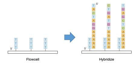
3. Template registration: Once hybridized, a "Fill & Lock" step fills up the rest of the open bases from the Poly-A tail followed by the addition of fluorescently labeled nucleotides to the start of the strand. A laser illuminates the flow cell and the camera records the location of each captured sample strand. The flow cell is moved in sequential steps to allow the camera to cover its entire active area. The dye molecules are then cleaved and washed away.
