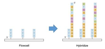
3. Template registration: Once hybridized, a "Fill & Lock" step fills up the rest of the open bases from the Poly-A tail followed by the addition of fluorescently labeled nucleotides to the start of the strand. A laser illuminates the flow cell and the camera records the location of each captured sample strand. The flow cell is moved in sequential steps to allow the camera to cover its entire active area. The dye molecules are then cleaved and washed away.
